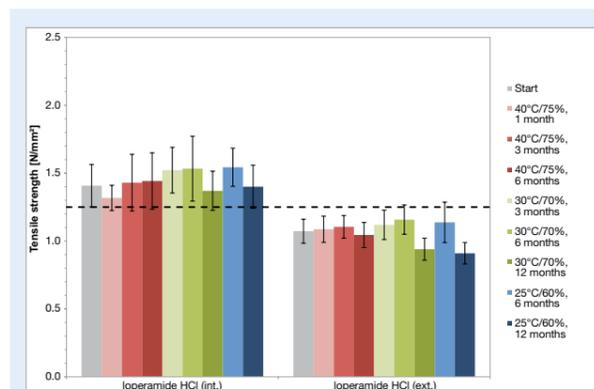
Figure 4. Tensile strength of the ODT formulations as function of storage time and condition (mean values (n=20), ±SD).
