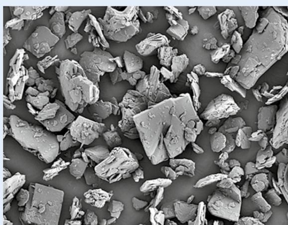
Figure 1. Scanning electron microscopy (SEM) image of loperamide HCl (SE, 5 kV).
