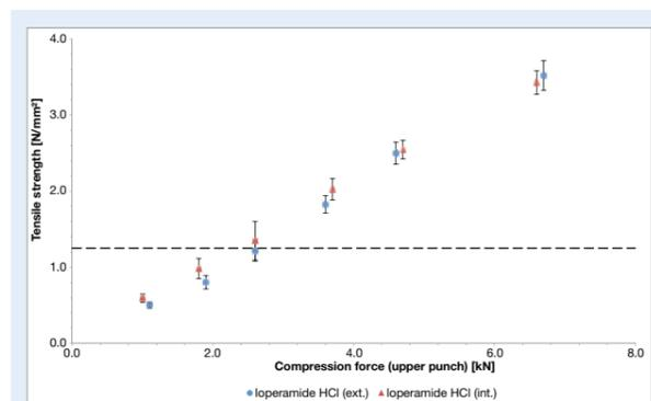
Figure 2. Tensile strength of the two ODT formulations as function of compression force (mean values (n=20), ±SD).
