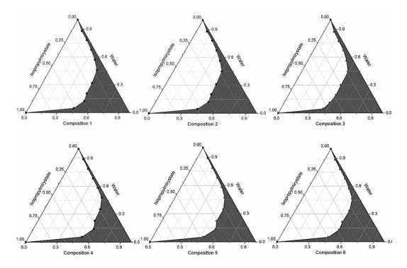
Figure 1. Pseudoternary phase diagrams of compositions 1–6, (Shaded areas represented microemulsions).
