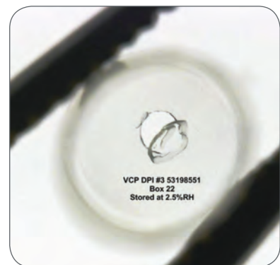
Figure 10: Vcaps ® Plus capsule dome after puncturing in a DPI
