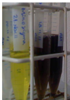
Fig. 5 Photo of minocycline solutions: a just-prepared (in yellow) and after one-week, in PBS, evidencing degradation (in brown).
