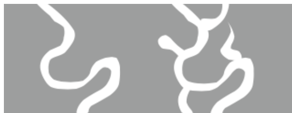
Fig. 9 Schematic representation of a pore structure evidencing a curved, tortuous single path from bottom surface to upper surface (left); a tangle of curved pores with intersections and dead ends (right) (adapted from Siegel, 2012).
