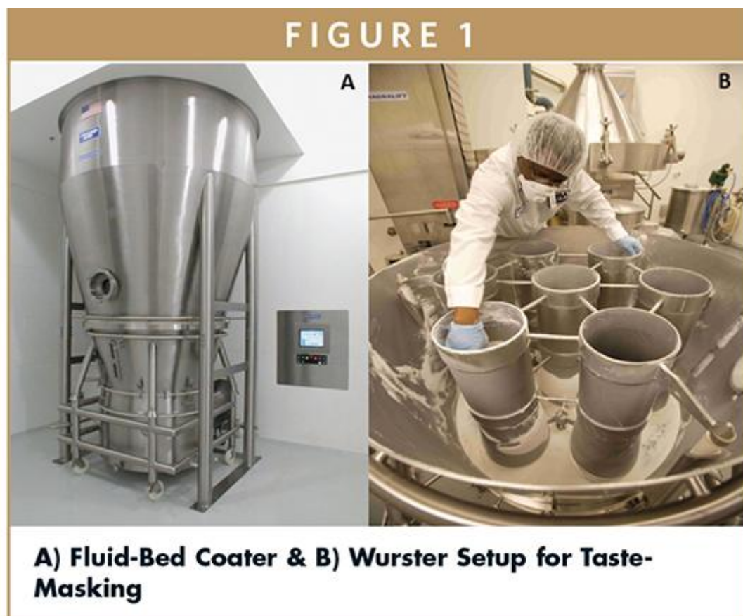
Figure 3:- Fluid –Bed Coater & Wurster setup for taste masking.
