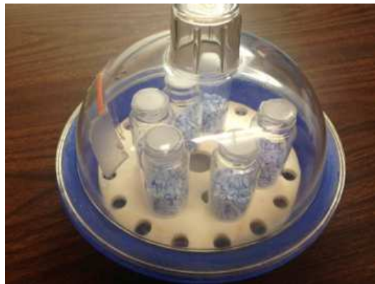
Fig 3.5A(Right): Colored indicator and glass vial used for permeability test; Fig 3.4B(Left): the 75% humidity controlled desiccator containing vials with films glued on top which created a constant humidity difference and provided a constant driving force for vapor transmission.
