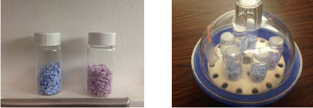
Fig 1.6a (L): Colored indicator and glass vial, the blue means the desiccants were dry and red indicated it was moisture absorbed so no longer good for usage; Fig 1.6b (R): 75%RH humidity controlled desiccator containing vials with films glued on top. Each experiment was repeated with n=6 .
