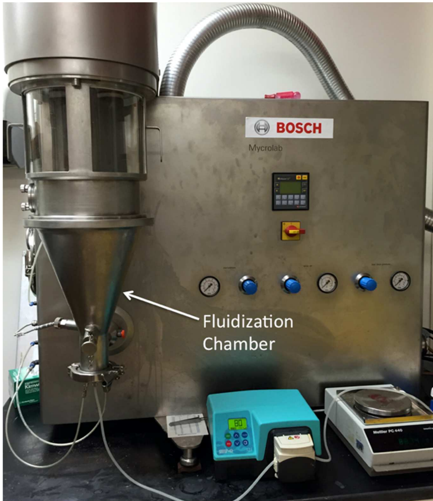
Fig 1.8. The set up of the Bosch Mycrolab fluid bed coating equipment. The Pump and balances was also needed for the coating process
