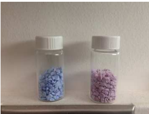
Fig 3.5A(Right): Colored indicator and glass vial used for permeability test; Fig 3.4B(Left): the 75% humidity controlled desiccator containing vials with films glued on top which created a constant humidity difference and provided a constant driving force for vapor transmission.
