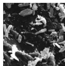
Example of an adhesive mixture of Lactohale® and salbutamolsulphate.
