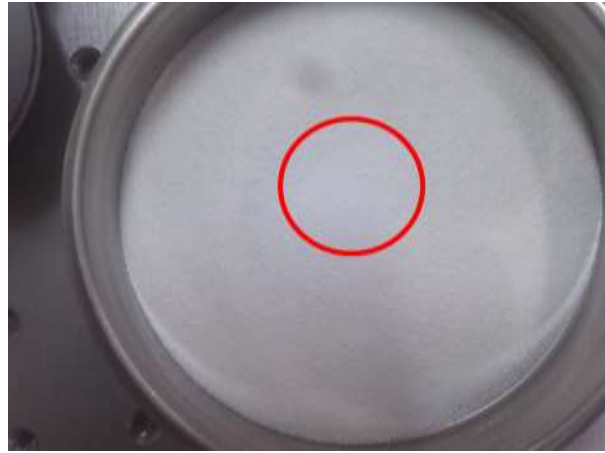
Figure 35 Mixture of 50% (w/w) sugar spheres and Cellets ® of nominal size 200 \mu\text{m} at the end the of the blending.
