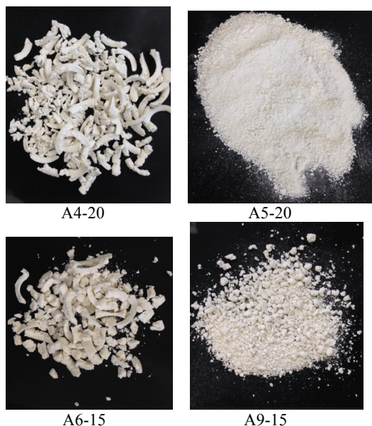
Figure 4. Photos of granules exiting with different molecular weight HPMC binders (see Table 4)
