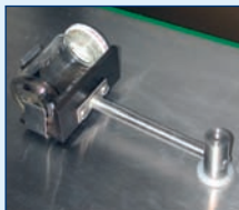
Friabimat™ used for testing the friability of pellets
