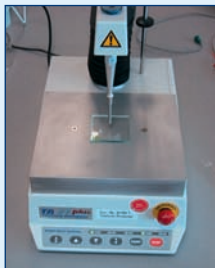
Texture Analyser™ used for testing the hardness of pellets
