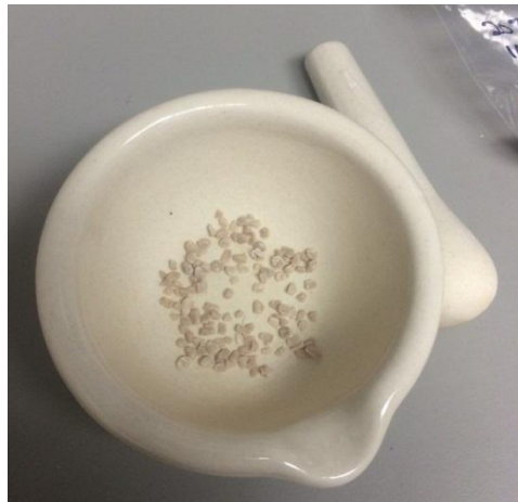
Figure 4.4: Mortar and Pestle approach for size reduction of multiparticulates.
