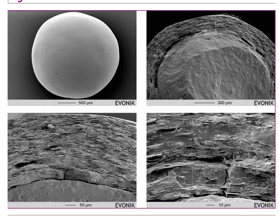
SEM images of the EUDRAGIT® coated final pellets showing the surface (top left) and cross-section (top right and both bottom images)
