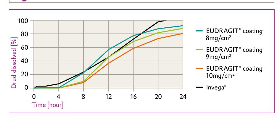
Dissolution profiles of paliperidone pellets with EUDRAGIT® coating compared to Invega® at pH 1.2
