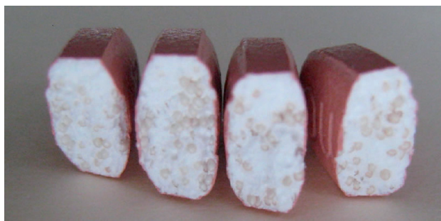
FIGURE 1: PELLET STRUCTURE APPARENT IN BROKEN MUPS® TABLETS.
