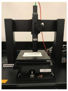
The gloss level of sample tablets was measured using a Model 805A Gloss/Surface Analysis System (Tricor Systems, Inc., USA). The quantity of light reflected at a 60° angle is reported as gloss units (GU) (Figure 3).
