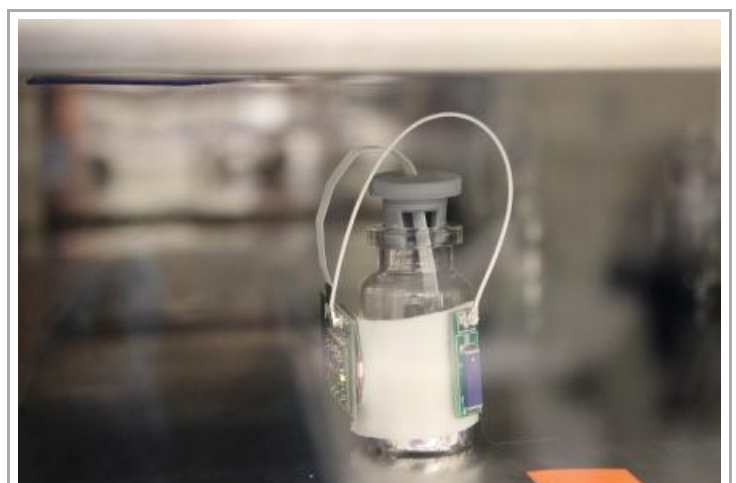
A wireless sensor developed to collect real-time data of the freeze-drying process. (Image provided by Jennifer Gray)
