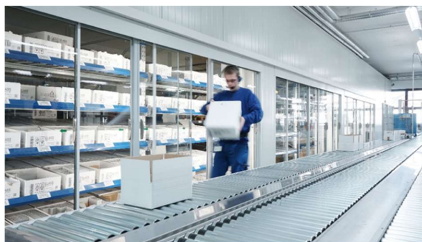
Figure 2: Cool products (2 – 8 °C) fully integrated into high-speed commissioning line
