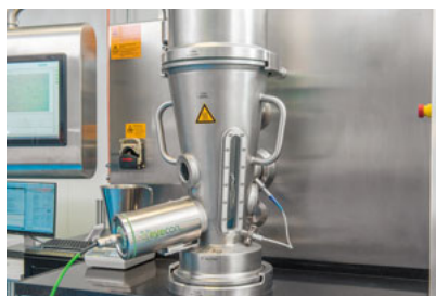
Figure 1: Process analytical technology compatible product container with Eyecon2 Particle Analyzer (Innopharma Technology). All figures are courtesy of the authors.
