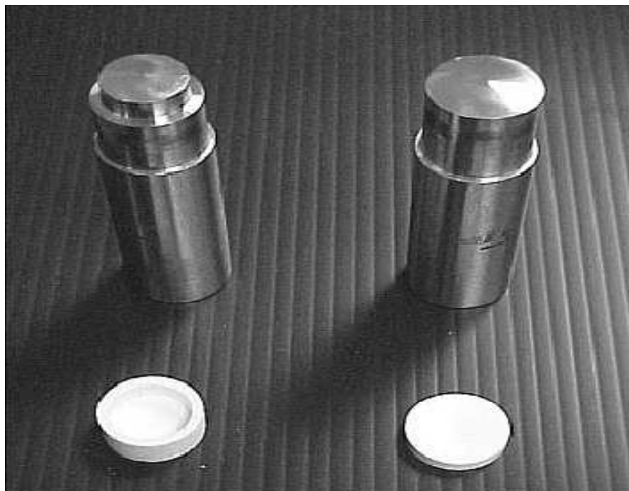
FIGURE 7 : PHOTO OF THE TOOLING USED TO DEMONSTRATE PROOF-OF-CONCEPT, A CUP, AND A FINISHED DOSAGE FORM
