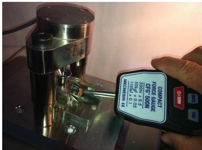
Using a handheld gauge to measure detachment (take-off) force on a benchtop tablet press and material tester
